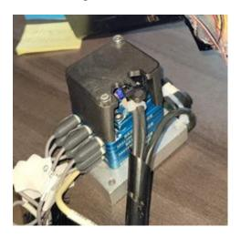
Figure 4: DTS Slice Micro DAQ
