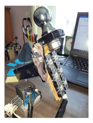
Figure 5: Strain Gauge Placement
