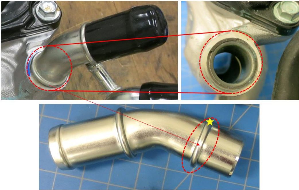
Figure 1: Installed tube (left), Cracked tube (right), Press-fit tube (bottom)
