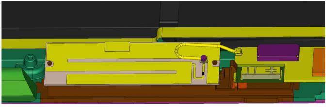
Figure 6: The GPS and Wi-Fi antennas.
