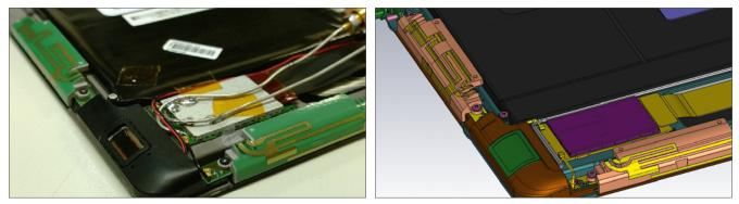
Figure 4: A physical prototype of a tablet with several antennas (left) and the equivalent simulation model (right).
