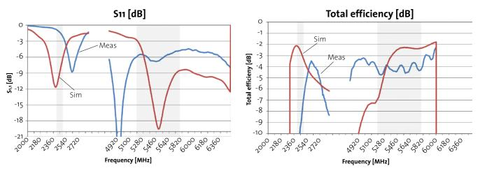
**Figure 2:** Uncertainties in material properties and component values leads to variation between the virtual prototype and the measured data (here for the Wi-Fi antenna). This means that accuracy is paramount in material characterization.
