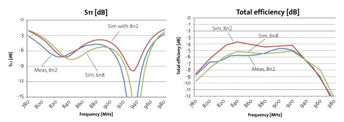
**Figure 3:** Simulated and measured S11 (top) and radiation efficiency (bottom) of the primary cellular antenna for two different matching circuit configurations. Tuning component values and material properties against measurement allows much better agreement to be achieved.
