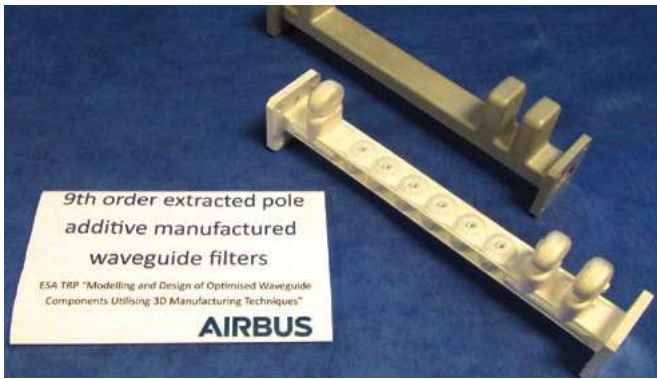
3D printed filters made by the Space Systems division of Airbus Defence and Space for the European Space Agency. Image courtesy Airbus Defence and Space.
