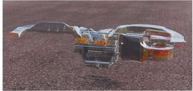
Turbulent flow structures in the 7 series HVAC.
