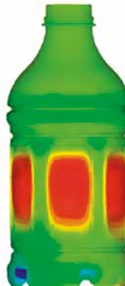
This Abaqus simulation clearly illustrates side panel displacement when a rigid plastic bottle is subjected to pressure.
