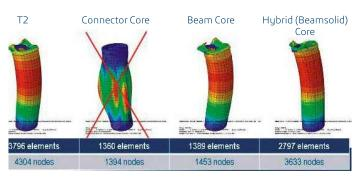
These Abaqus simulations illustrate the effectiveness of using different core materials for battery cell construction—here, the results of a modal study showing the first mode of vibration for different meshing strategies. For instance, the crossed out "Connector Core" model does not constrain the casing well and as such, its first mode of vibration introduces an unrealistic vibration, i.e. at a very low frequency, clearly visible in the casing of the cylindrical battery cell.
