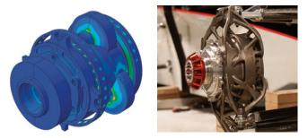
Stresses in gearbox assembly (left) where effect of bearing model, preload and loads are visualized. Gearbox assembled inside the upright (right).
