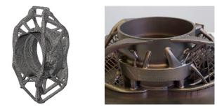
Topology optimization of the front upright in Tosca (left) was performed prior to preparation for 3D printing. The 3D-printed, left-rear upright before support removal and post heat treatment and prior to finishing via machining (right). The final product weighs a little more than a pound (545grams).
