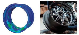
Optimization of the wheel shell (left) required over 4,000 iterations in Abaqus and two days of compute time, the majority of which was automated via Isight. Complete rim mounted with CRFP shell and aluminum center (right).
