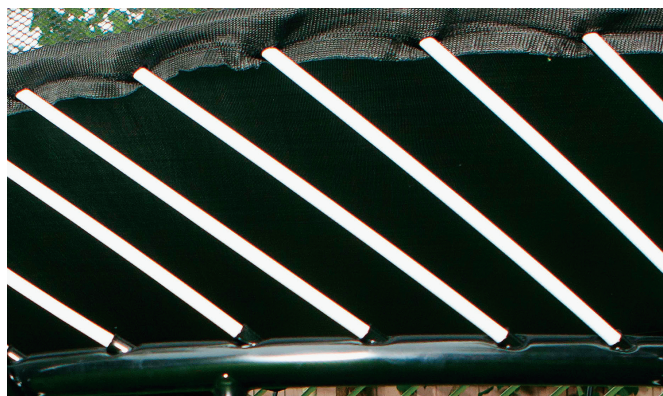
Figure 1. Closeup of the innovative support structure of a Springfree trampoline shows how white rods connect via cleats to the upper, soft-edged jumping surface. Lower end of rods attach to the secure metal frame that sits on the ground. Protective netting not shown.
