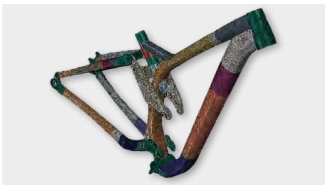
This Abaqus model of a Trek full-suspension mountain bike depicts solid and shell elements linked with constraints and connectors, a welded butted aluminum frame, and a magnesium rocker link.
