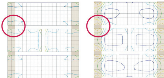
The masonry on the left was repointed with compatible mortar, the one on the right with mortar of greater rigidity. Note the stress lines extending into the structure—these will eventually crack or even crush the legacy material, leading to structural failure of an important artifact.
