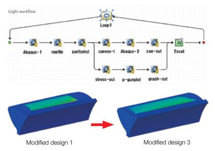
Optimizing gears with Isight resulted in a design that lowered contact stress across the entire surface.
