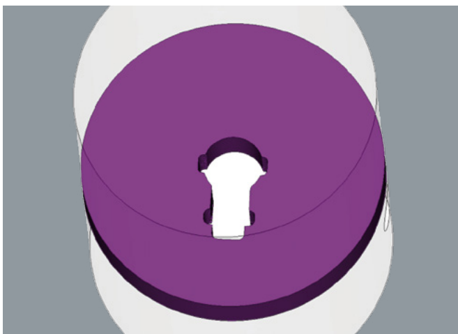
An initial design space for a winch gear support plate optimization exercise. Designs that stay with such a flat, circular shape can be susceptible to warping under the high stresses of competitive sailing.
