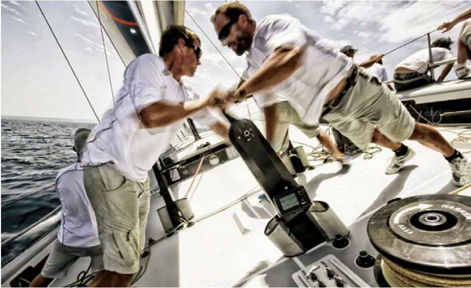
A two-sailor team quickly rotates the "coffee grinder" that powers the gear driving a winch (lower right).
