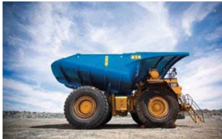
The dump truck tray extends over the driver's cab and can be as long as the entire vehicle.
