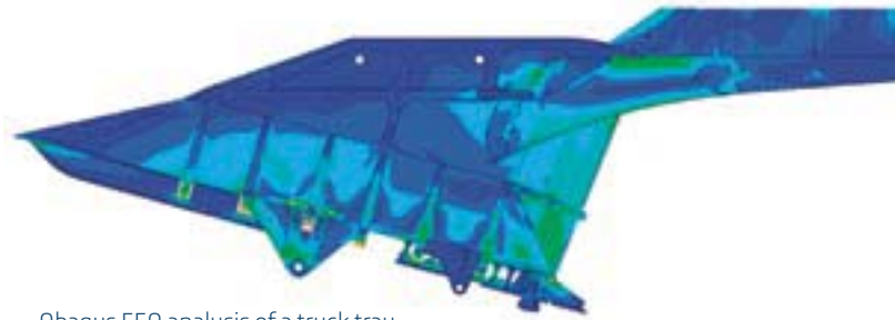
Abaqus FEA analysis of a truck tray.
