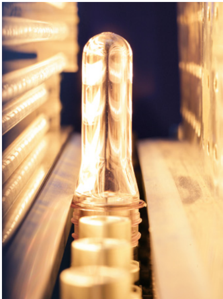
A preform of molten PET plastic (with thin stretch rod visible inside), en route to a blow mold where it will be injected with air to expand it into a plastic bottle.
