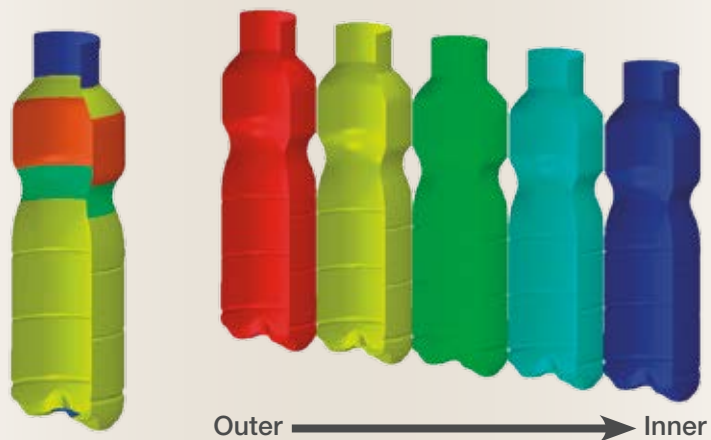
The heat transfer method is an alternative analysis available in Abaqus.
