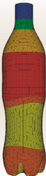
An example of a CO 2 loss rate analysis in Abaqus. A greater proportion of the gas passes through the thinner areas of the bottle.
