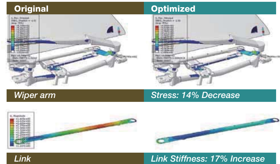
Figure 2. Comparison of FEA results for wiper arm and link before and after optimization.
