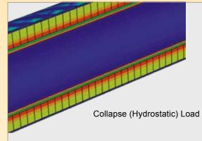
(Top) Cross-section analysis of a portion of DeepFlex pipe with stress distribution registered during collapse testing.
