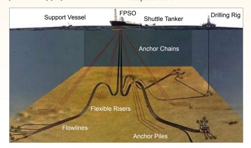
Diagram showing intended applications of DeepFlex pipe in deepwater installations. All-composite flexible fiber-reinforced pipe can be used for dynamic risers, subsea flowlines and pipelines, subsea jumpers, and surface jumpers on hybrid risers or on platform decks.
