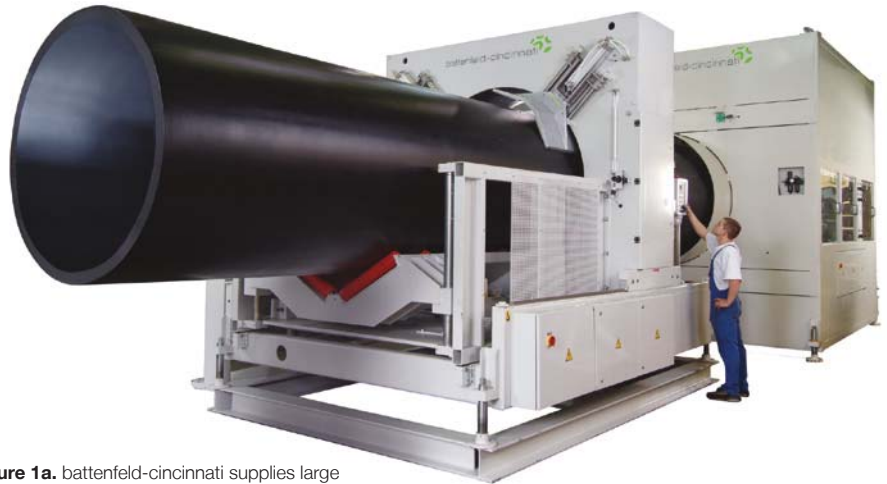
Figure 1a. battenfeld-cincinnati supplies large diameter pipe lines with diameters up to 2.6 m (photo © battenfeld-cincinnati)
