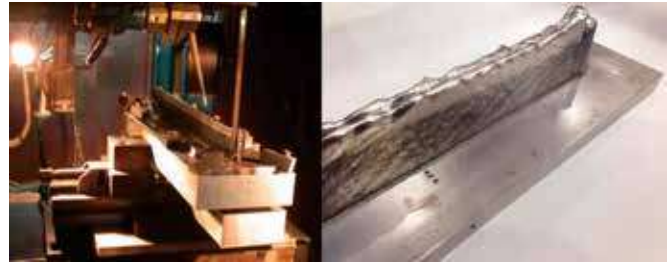
Figure 6. Wire EBAM test set-up (left) and example of W-EBAM test piece.
