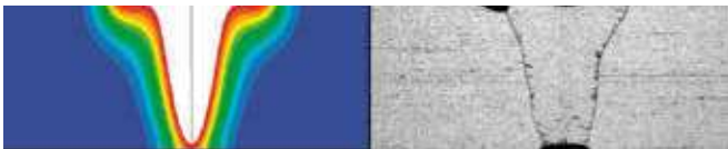
Figure 1. Conventional welding simulation comparing fusion zone size and shape.
