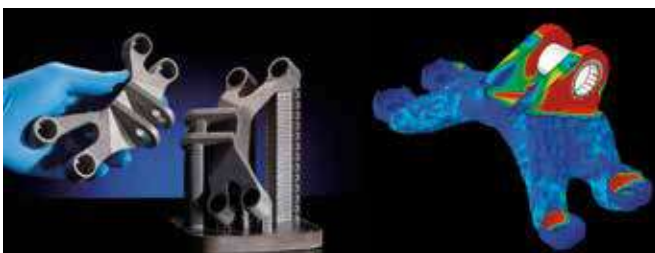
Figure 3. SLM part designed using Tosca topology optimization and produced using the SLM process 2 .
