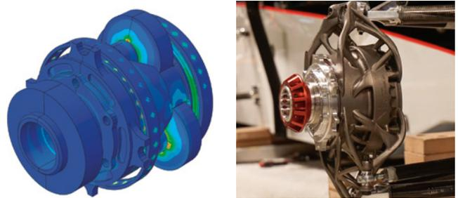
Stresses in gearbox assembly (left) where effect of bearing model, preload and loads are visualized. Gearbox assembled inside the upright (right).
