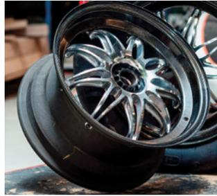
Optimization of the wheel shell (left) required over 4,000 iterations in Abaqus and two days of compute time, the majority of which was automated via Isight. Complete rim mounted with CRFP shell and aluminum center (right).
