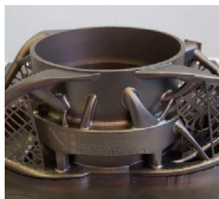
Topology optimization of the front upright in Tosca (left) was performed prior to preparation for 3D printing. The 3D-printed, left-rear upright before support removal and post heat treatment and prior to finishing via machining (right). The final product weighs a little more than a pound (545grams).
