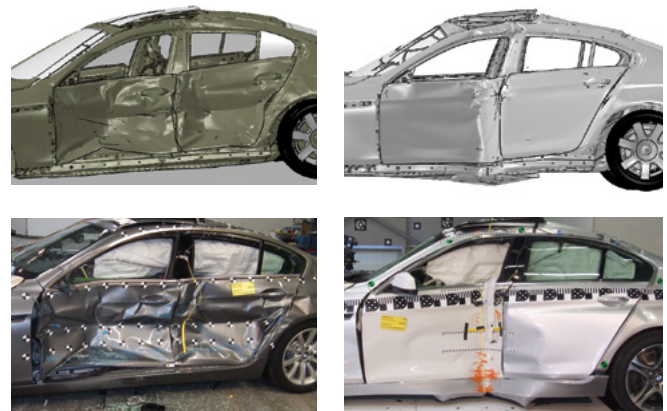
Figure 3. Side impact load cases are often the most difficult from a crashworthiness perspective. The figures above show actual BMW 6 Series Gran Coupé results for two standard side crash tests: IIHS side impact with moving deformable barrier (left); and FMVSS 214 side pole impact (right). For each, the corresponding design simulation results are also shown which accurately predicted the passive safety performance and led to the zero-prototype success.
