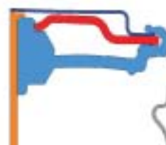
Internal pressure is applied until de-crimping occurs.
