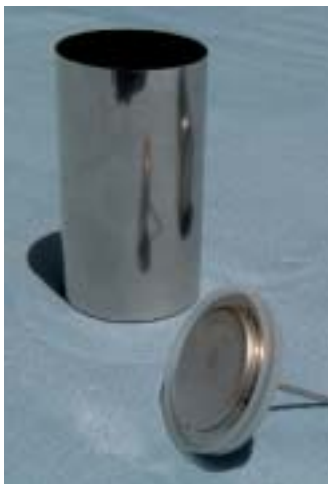
The initial state of the battery can with no groove.
