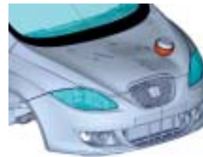
Simulation of adult headform over full vehicle. (Courtesy of SEAT)
