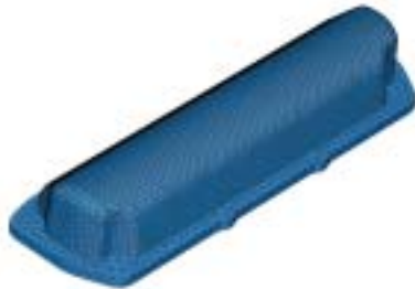
Acoustic infinite element model for a geometrically simple engine valve cover.
