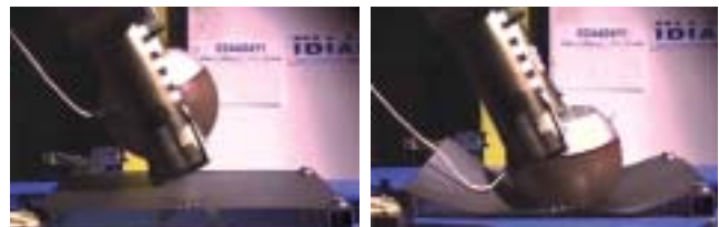
Physical test of the adult headform impactor.
