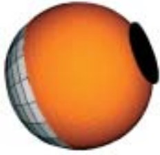
FE model of the adult headform generated for certification tests.
