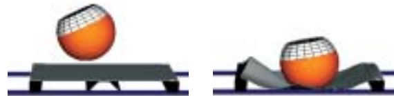
Realistic simulation of the adult headform impactor.
