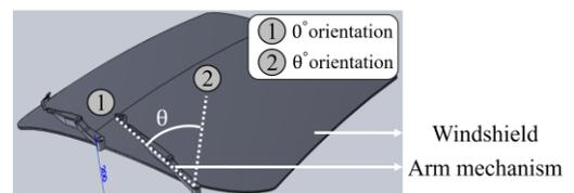
Fig. 3 A schematic of the compression force estimation on windshield
