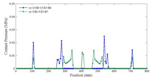
Fig. 8(a) Simulated pressure distributions under the optimization procedures based on IND1
