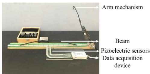
Fig. 1 A schematic of the experimental set-up
