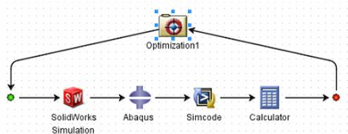
Fig. 4 A flowchart of the optimization procedures
