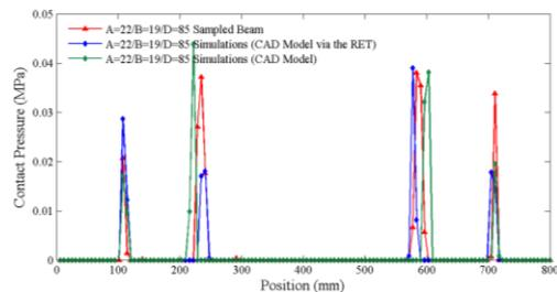
Fig. 9(c) Pressure distributions of the sampled beam, the CAD model of the beam via the reverse-engineering technology, and the CAD model of the beam based on  $A=22/B=19/D=85$
