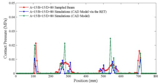
Fig. 9(a) Pressure distributions of the sampled beam, the CAD model of the beam via the reverse-engineering technology, and the CAD model of the beam based on  $A=15/B=15/D=80$
