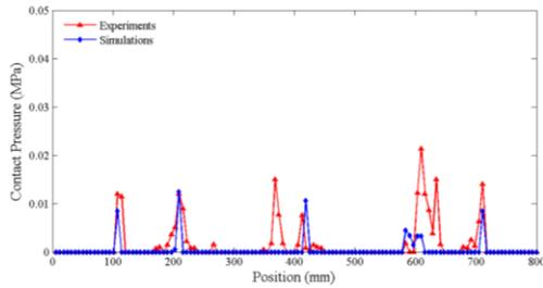
Fig. 6 Comparisons of the pressure distribution based on the experiments and the simulations
