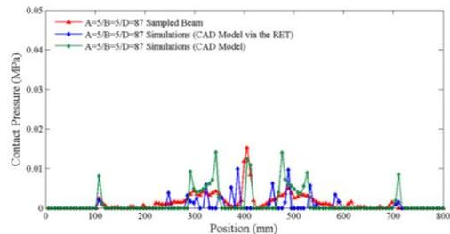
Fig. 9(b) Pressure distributions of the sampled beam, the CAD model of the beam via the reverse-engineering technology, and the CAD model of the beam based on  $A=5/B=5/D=87$
