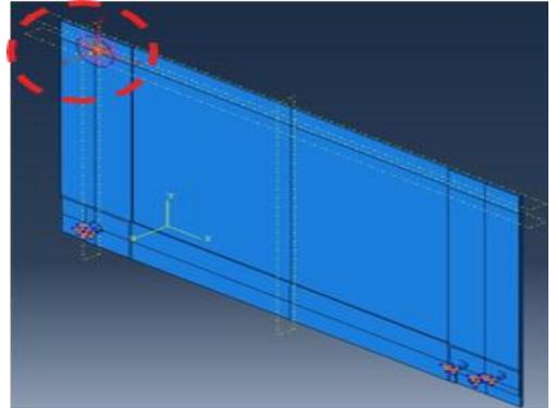
Figure 5, Load and B.C.'s for all fifteen CAE models
