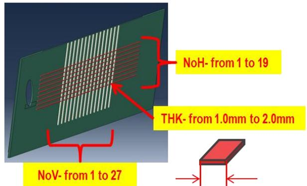
Figure 3, Three design factors in optimizing the folded stand
