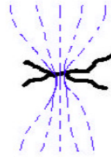
Constriction in Current flow due to Asperities
